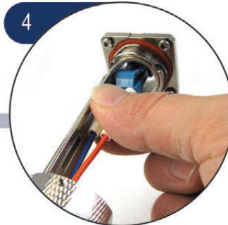
4 Mate LC connector to adapters
