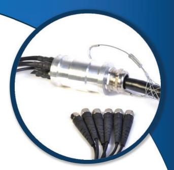
An outdoor heat shrink divider splits fiber cables into separate ruggedized short branches equipped with fiber optic outdoor harsh environment connectors. The connection to the RRH is ensured with factory terminated Fiber jumpers with RRH interface (large range available to fit most of RRH in the market). An alternative system with metal canister is available. The metal canister provides a secure and reliable hoisting and grounding mechanism.
