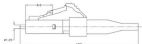
LC Duplex Connector with 900µm Boot
