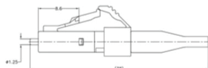
LC Duplex Connector with 900µm Boot
