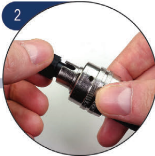
2 Carefully remove MPO dust cap
