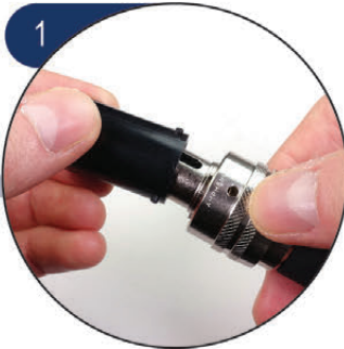
1 Twist and remove PT-MPO dust cap
