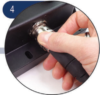
4 Twist coupling sleeve 1/4 turn until audible "click"
