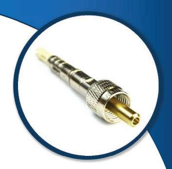
The connector ferrules is made from Beryllium Copper allowing the ferrule to act as a heat sink, pulling the heat quickly away from the fiber, when used. Damage threshold on these types of connectors will vary based on launch conditions and operational wavelength. The front body of the connector is a Beryllium Copper ferrule that is designed with a custom, high-tolerance, application-specific hole diameter.
