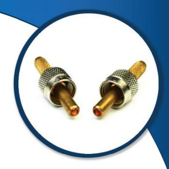
Damage threshold on these types of connectors will vary based on launch conditions and operational wavelength. The front body of the connector is a Beryllium Copper ferrule that is designed with a custom, high-tolerance, application specific hole diameter.
