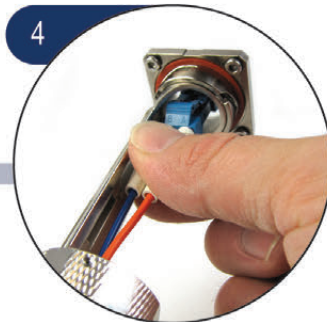
Mate LC connector to adapters
