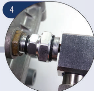
4 Align coupler to coupling fitting
