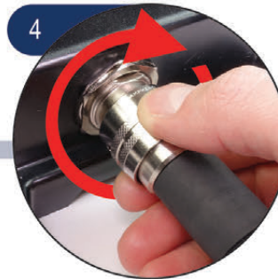
4 Twist coupling sleeve 1/4 turn until audible "click"
